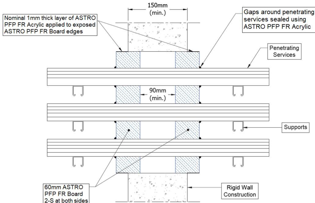
**A.1.7.1 Two side penetration seal with cables**
