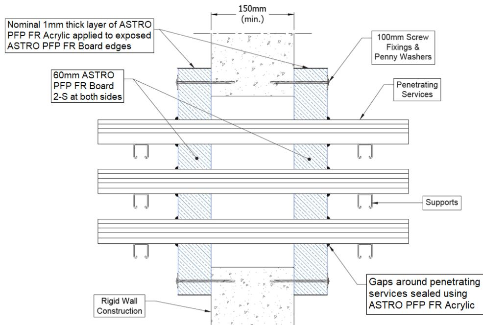
**A.1.8.1 Two side penetration seal with cables**
