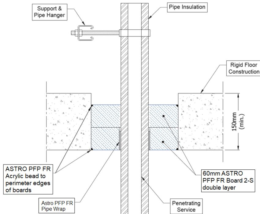
**A.3.9.1 Back to back penetration seal with pipes**
